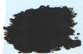
Hematite is weighting material used to increase the density of drilling fluids to control formation pressures. It has a specific gravity of 4.8 and can be used to increase the density in oil and water-based drilling fluids It has a higher specific gravity than barite, and so requires less total product to achieve the same fluid density.
