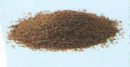
Walnut ground shells are used to help combat lost circulation in water-based and non-aqueous fluids. Walnut Shell is available in three grades: fine, medium, and coarse. All three grades may be used in pills for spotting opposite thief zones and in high filtration squeeze slurries. Walnut Shell can be used in the active mud system to help prevent lost returns.
